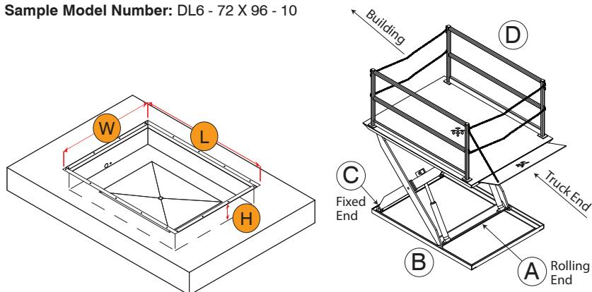
\* Capacities are based on evenly distributed loads. Single axle rolling load capacity is 80% of rated capacity across the ends and 50% of rated capacity across the sides - based on model.
